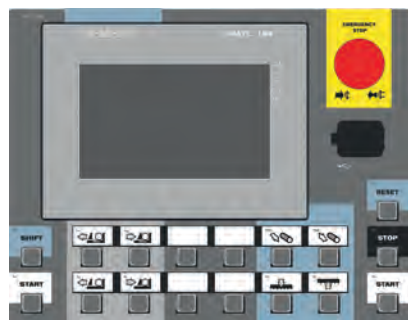
CONTROL PANEL: SIEMENS (X-CNC)
